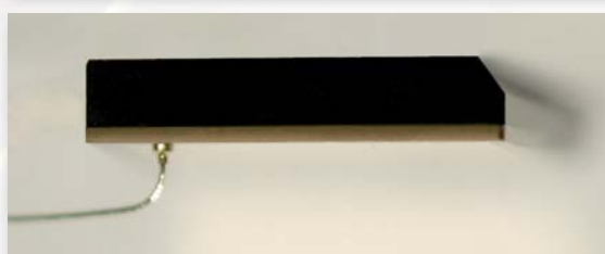
Sensing element of ionizing radiation detector made of CVD single crystals doped with diamond substrates
