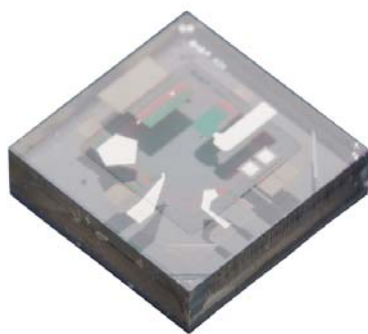
HBAR with a diamond single crystal as a substrate with complex electrodes geometry
