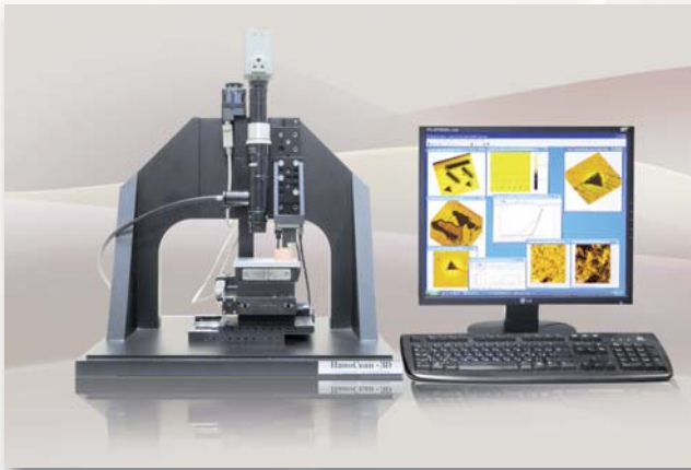
Scanning nano-hardness tester NanoScan-3D
