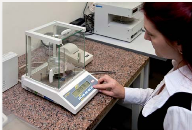
Electronic scales (Kern) with attachment (Sartorius)
