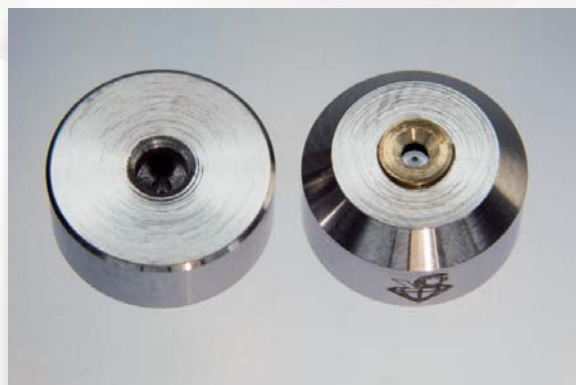
Nozzles in an assembly with a working part of a diamond single crystal
