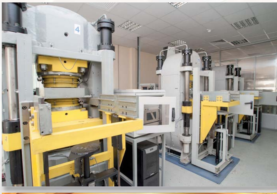
Universal high-pressure growth units (model URS-01/V).
