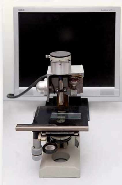
High-frequency acoustic microscope (range 25–100 MHz)
