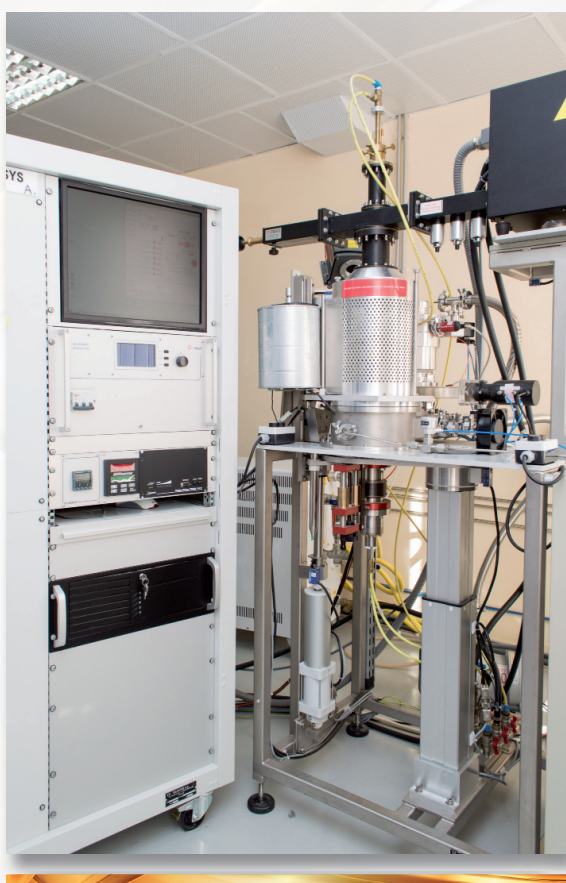
Plassys BJS 150 diamond deposition reactor
