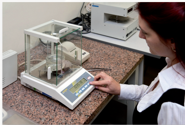
Electronic scales (Kern) with attachment (Sartorius)
