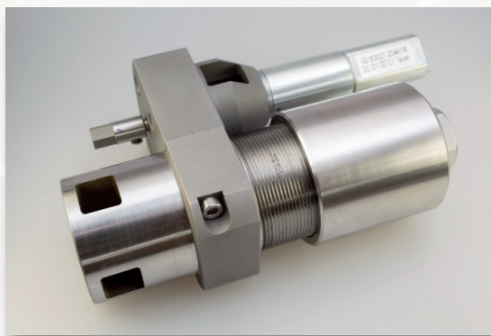
Shear diamond anvil cells with electric drive developed and produced by TISNCM
