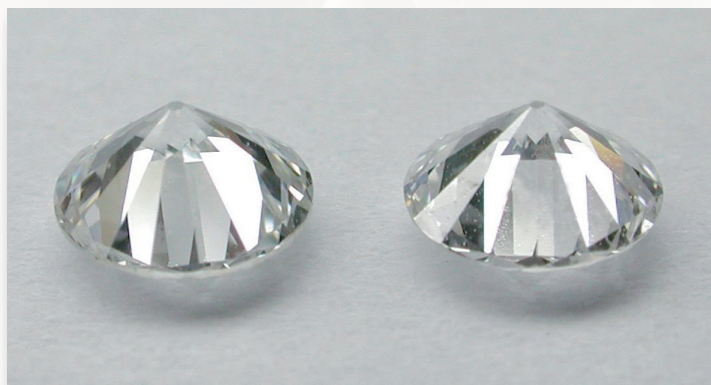
Anvils of high-purity diamond single crystals
