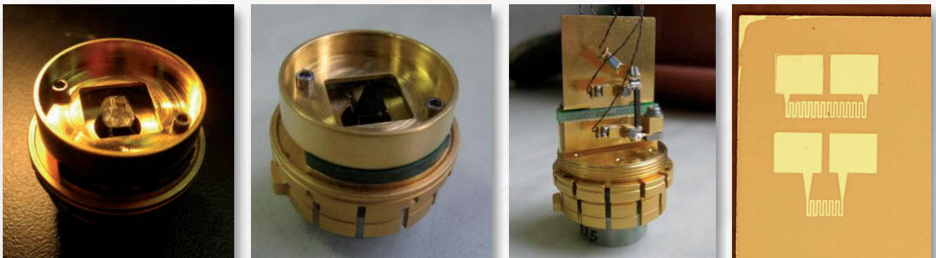
Studied structures in the holders for studying the heat capacity and thermal conductivity of diamond
